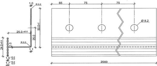
Vertical connection profile – " Brillux WDVS ALU-Verbindungsleiste 3580" (dimensions in millimetres)
